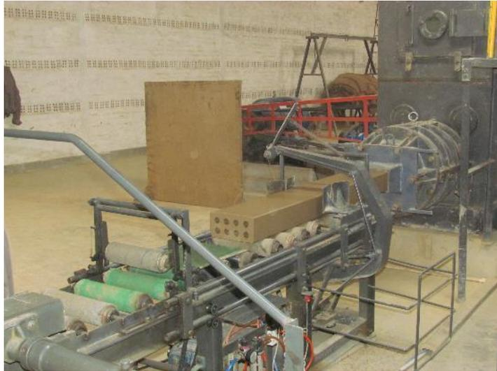
The extruded slab is wire-cut to get individual green bricks.
