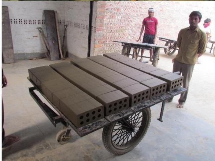
The moulded bricks are dried in the drying shade before loading these into the kiln for firing. The drying time varies with the weather conditions – 15-20 days in summer months while 30 or more days in winter months.
