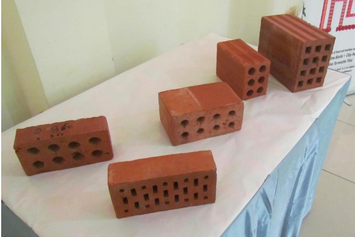
Figure 1: Various types of perforated bricks
