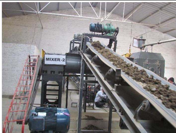
The clay mix is then fed into the vacuum extruder which produces perforated slab through extrusion.
