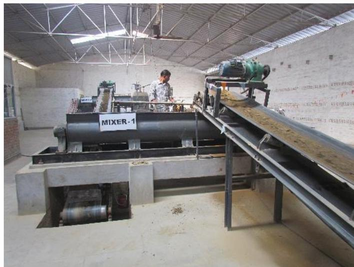
To get a proper homogeneous clay mix, the clay is again passed through a second mixer just before the extruder.
